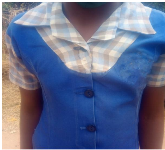
Figure 2: Unproportioned panels and distorted yoke shape.
