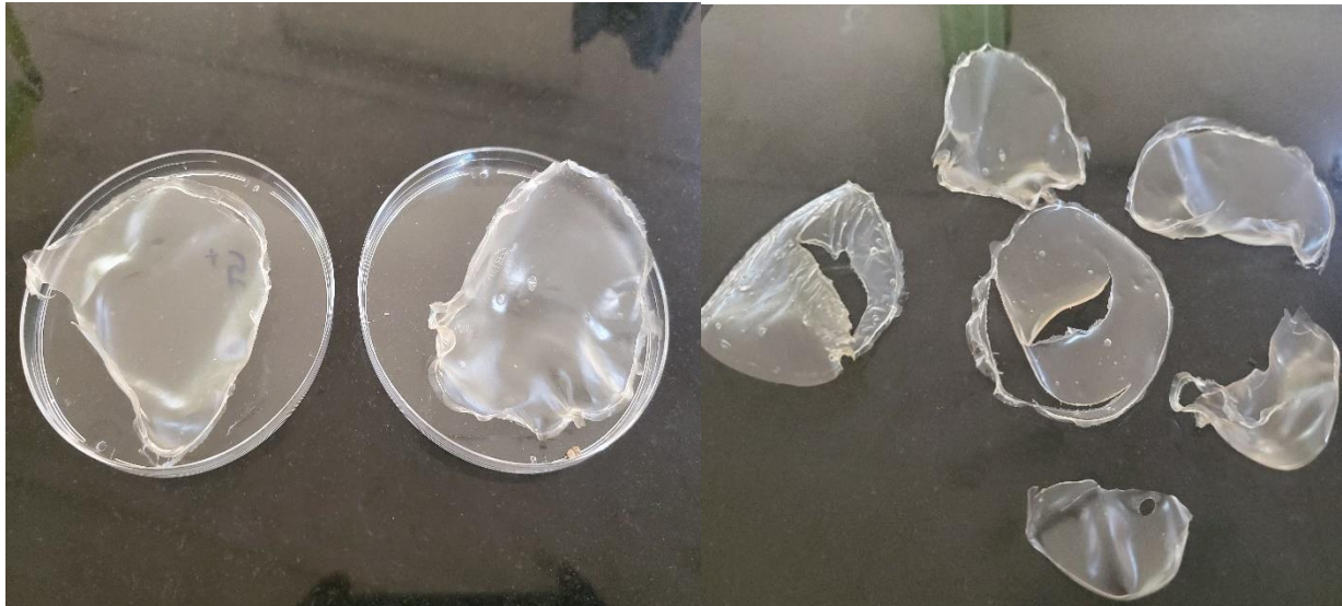
Figure 4. 1shows biodegradable plastic samples produced from mushroom starch after drying
