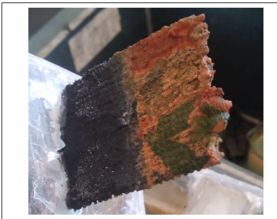
Figure 5.1: Shows rust and algae on the anode electrode of Double Chamber MFC
