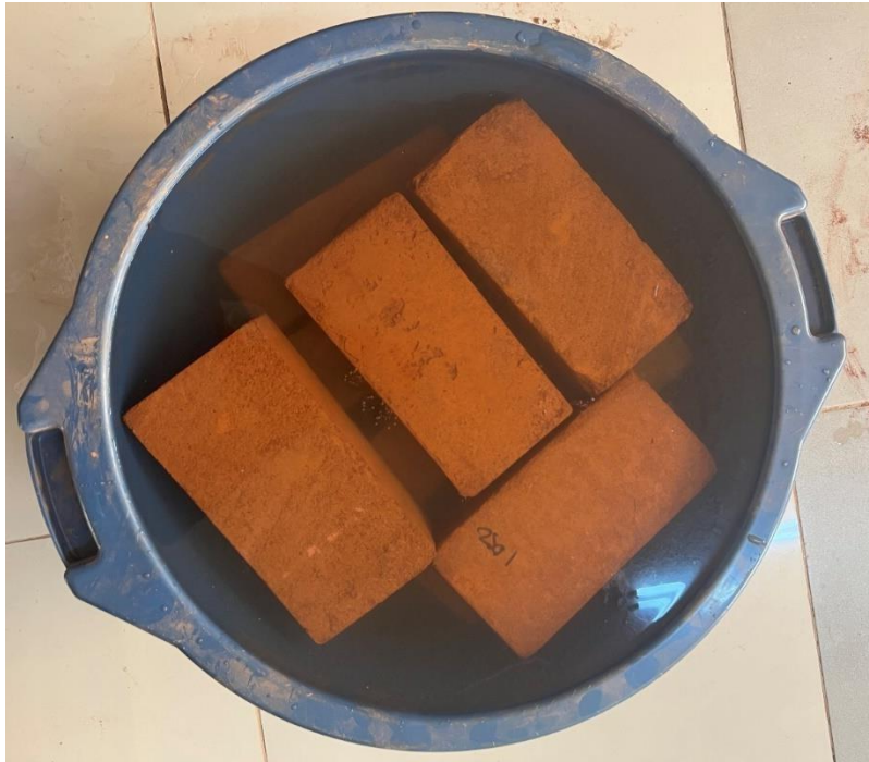
Figure 3.12: Water Absorption Test
