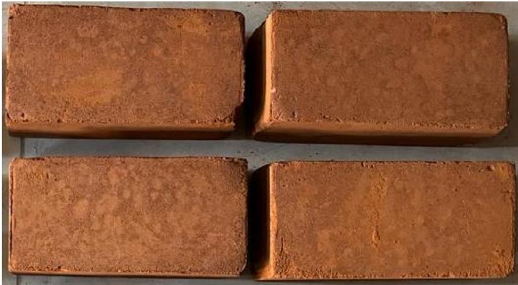
Figure 4.8: Sample Bricks Fired at 950 °C
