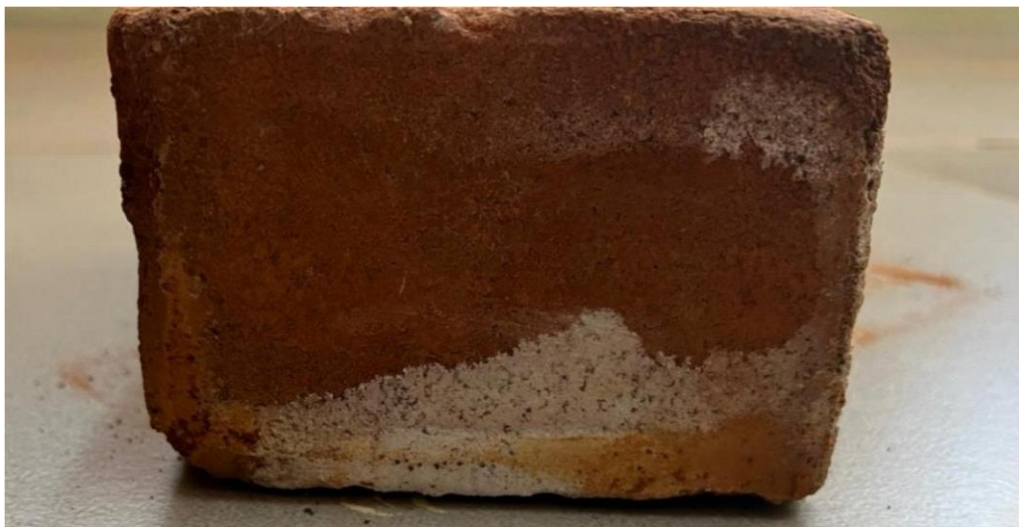
Figure 4.16: Brick Efflorescence at 50 wt.% Combination
