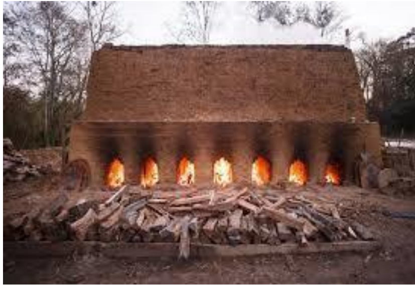
Figure 2.6: Clamp Burning (Civil Engineers PK, 2016)
