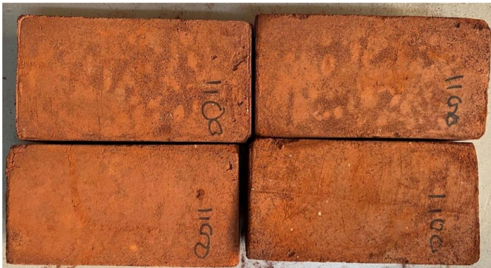
Figure 4.9: Sample Bricks Fired at 1100 °C
