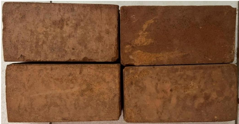
Figure 4.7: Sample Bricks Before Firing
