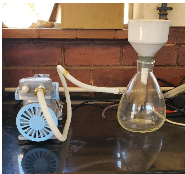
Figure 3.4 | Vacuum filtration apparatus to obtain E.goetzei seed extracts coagulant solution
