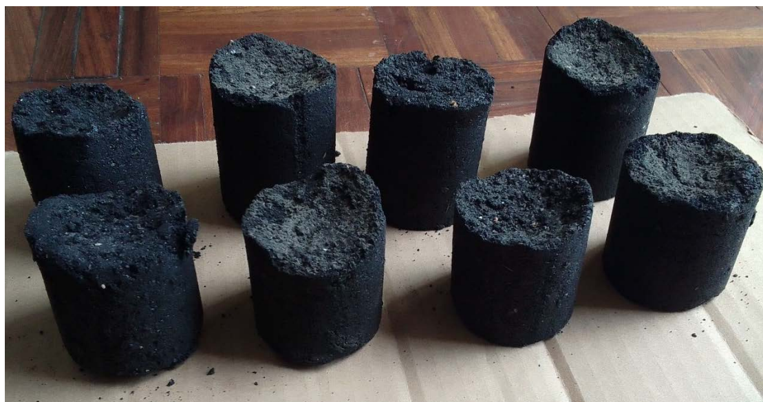
Figure 4.6. Briquettes produced using coal fines, Kaolin clay and Molasses
