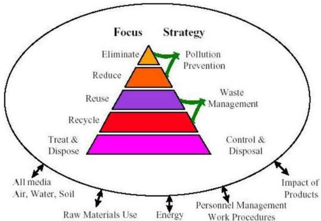
Fig 2.7 An Integrated Approach to Cleaner Production (Gavrilescu, 2003)
