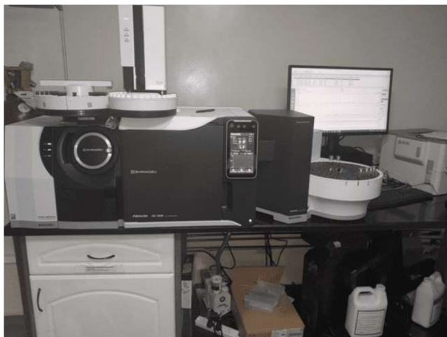
Fig. 2 Shimadzu Nexis GC2030, GCMS TQ8040NX Triple Quadrupole Mass Spectrometer, HS-20NX mode. Source (This study)
