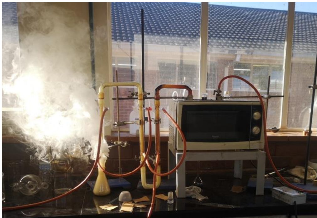
Figure 4.3: Microwave-assisted pyrolysis experimental setup
