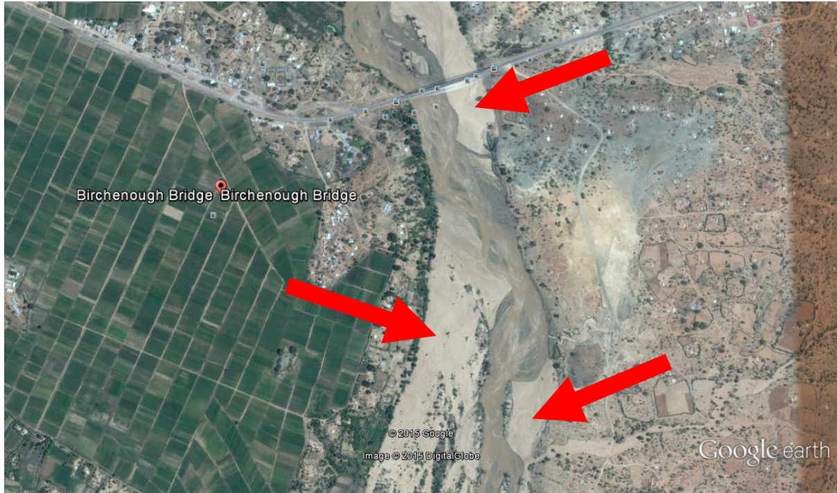
Fig. 9.6: Siltation along the Save river and its tributaries (red arrows showing areas of sediment deposition) (Source: Google Earth)
